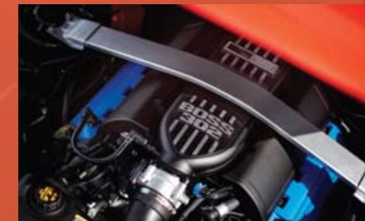
**“Runners-in-the-box”** intake plenum enhances airflow for charges to the redline
